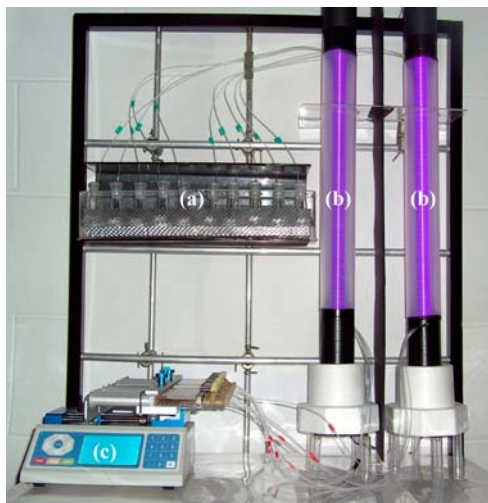
Figure 1. Multimicrocapillary flow reactor (M \mu CFR): (a) collection flasks; (b) FEP microcapillaries; (c) 10-syringe pump.
